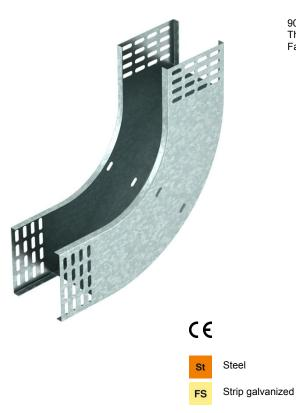
90° rising vertical bend, for all cable tray types of 110 mm side height. The vertical bend is pushed over the end of the cable tray and screwed tight. Fastening materials should be ordered separately.
