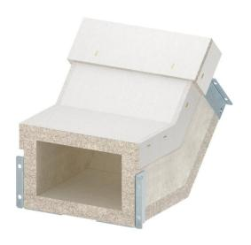
Vertical bend, rising, for PYROLINE® Con S El60 fire protection duct, type PLCS D061220, consisting of fibreglass light concrete which is resistant to water and frost for the creation of vertical changes of direction (45°) of the duct. Mounted connectors ensure quick mounting in situ, whilst loosely placed covers ensure quick inspection and reassignment.
