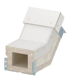
Vertical bend, rising, for PYROLINE® Con S El60 fire protection duct, type PLCS D060810, consisting of fibreglass light concrete which is resistant to water and frost for the creation of vertical changes of direction (45°) of the duct. Mounted connectors ensure quick mounting in situ, whilst loosely placed covers ensure quick inspection and reassignment.
