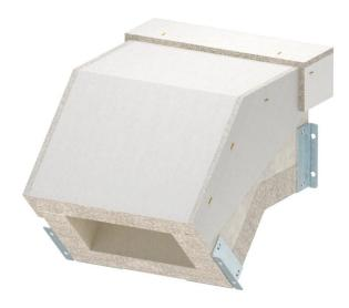
Vertical bend, falling, for PYROLINE® Con S El90 fire protection duct, type PLCS D091220, consisting of fibreglass light concrete which is resistant to water and frost for the creation of vertical changes of direction (45°) in the duct. Mounted connectors ensure quick mounting in situ, whilst loosely placed covers ensure quick inspection and reassignment.
