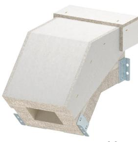
Falling vertical bend for PYROLINE® Con S EI90 fire protection duct, type PLCS D090810, consisting of fibreglass light concrete which is resistant to water and frost for the creation of vertical changes of direction (45°) in the duct. Mounted connectors ensure quick mounting in situ, whilst loosely placed covers ensure quick inspection and reassignment.
