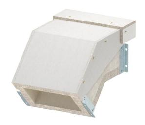
Falling vertical bend for PYROLINE® Con S El60 fire protection duct, type PLCS D061220, consisting of fibreglass light concrete which is resistant to water and frost for the creation of vertical changes of direction (45°) in the duct. Mounted connectors ensure quick mounting in situ, whilst loosely placed covers ensure quick inspection and reassignment.
