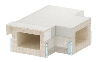
T piece for PYROLINE® Con S El90 fire protection duct, type PLCS D091220, consisting of fibreglass light concrete which is resistant to water and frost, for the creation of T branches in the duct route. Mounted connectors ensure quick mounting in situ, whilst loosely placed covers ensure quick inspection and reassignment.
