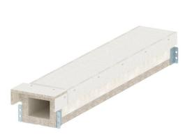
Fire protection duct made of water and frost-resistant fibreglass lightweight concrete of material class A1 according to EN 13501-1 for fireproof routing of cables in escape and rescue routes. El30 - El60 classification as installation duct according to EN 13501-2 on the basis of tests in accordance with EN 1366-5. When there is an internal fire load (cable fire), the duct prevents the spread of fire from one fire section to another.
