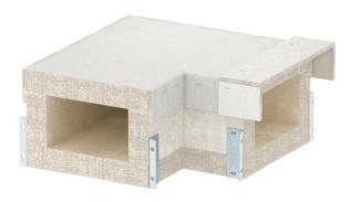
90° bend for PYROLINE® Con S El90 fire protection duct, type PLCS D091220, consisting of fibreglass light concrete which is resistant to water and frost for the creation of horizontal changes of direction in the duct. Mounted connectors ensure quick mounting in situ, whilst loosely placed covers ensure quick inspection and reassignment.
