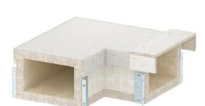
90° bend for PYROLINE® Con S El60 fire protection duct, type PLCS D061220, consisting of fibre glass light concrete which is resistant to water and frost for the creation of horizontal changes of direction of the duct. Mounted connectors ensure quick mounting in situ, whilst loosely placed covers ensure quick inspection and reassignment.
