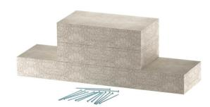
Wall connection collar for PYROLINE® Con D El90 fire protection duct, type PLCD D091220, consisting of fibreglass light concrete, which is resistant to water and frost, for mounting on the fire protection duct in the area of wall and ceiling connections and wall and ceiling penetrations. Consists of 3 single plates (width 100 mm, depth 40 mm). Including countersunk head screws. Including counter-sunk head screws.
