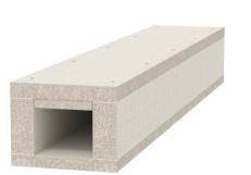
Fire protection duct made of water and frost-resistant fibreglass lightweight concrete of material class A1 according to EN 13501-1 for fireproof routing of cables in escape and rescue routes. El60 classification as installation duct according to EN 13501-2 on the basis of tests according to EN 1366-5. When there is an internal fire load (cable fire), the duct prevents the spread of fire from one fire section to another.
