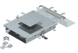
Ready-to-mount trunking extension unit with a device installation lid for the installation of an installation unit of nominal size 4, consisting of the trunking base (floor trough with side and floor covering guide profiles), trunking lid with blank mounting opening and a flushfloor end cover. The scope of delivery contains three height-adjustable wall fixing brackets, three screed anchors and trunking connection brackets.
