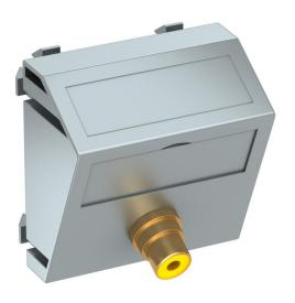
Multimedia support with one cinch connection socket for composite video, slanting cable outlet, with labelling panel, cinch socket (RCA) with soldered connection, colour coding yellow. Support plate with locking fastening, suitable for horizontal and vertical installation in the system environment.
