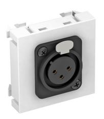
Multimedia support with one XLR connection socket, straight cable outlet, without labelling panel, 3-pin XLR socket with screw connection. Support plate with locking fastening, suitable for horizontal and vertical installation in the system environment.
