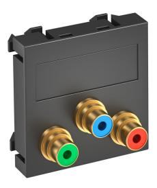
Multimedia support with three cinch connection sockets for component video, straight cable outlet, with labelling panel, three cinch couplings (RCA), socket-socket version, colour coding red/green/blue. Support plate with locking fastening, suitable for horizontal and vertical installation in the system environment.
