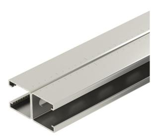
Heavy-duty Unistrut with continuous perforation in base, slot width 22 mm. Double version, i.e. two profile rails are interconnected on the base (welded).
