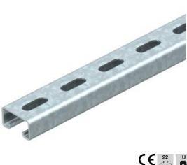
Heavy-duty C profile rail for individual installation of support constructions, e.g. for cable trays or as a panel for switchgear cabinets. Can also be used for cable routing, in conjunction with clamp clips with a U foot.
