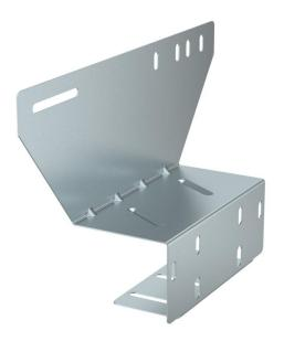
Universal mounting plate to fasten the FireBox T series to the front side of cable trays and mesh cable trays as well as cable ladders of max. 60 mm side height. Enables the secure mounting of cables that maintain electrical functionality, without having to bend it over the side rail. Suitable for all FireBoxes.
