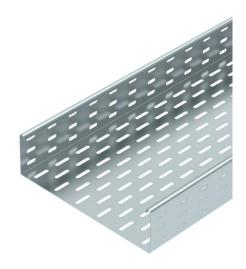
MKS 85 = medium-duty cable tray system with a side height of 85 mm. Including connector, type RLVL 85. Magnetic shield insulation without cover 20 dB, with cover 50 dB.
