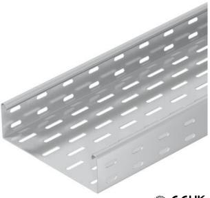
MKS 60 = Medium-duty cable tray system with a side height of 60 mm. Connecting parts should be ordered in the appropriate quantity. Magnetic shield insulation without cover 20 dB, with cover 50 dB.
