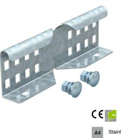
Angle connector as external connector to join cable ladders and fittings with a side height of 60 mm and continuous rail perforation. The bolt fastening ensures the continuity of the equipotential bonding.
