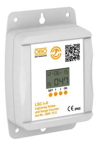
The LSC I+II lightning current meter measures and permanently saves pulse currents, together with the date and time. This ensures constant monitoring in order to notice if any lightning has struck the lightning protection system. Should this be the case, then the lightning protection system must be maintained according to VDE 0185-305 (IEC 62305).
