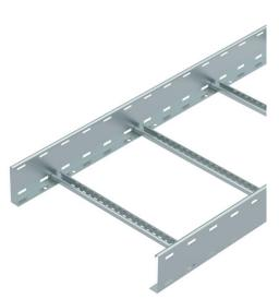
Cable ladder with perforated side rail of side height 110 mm with riveted C profile rungs, open in an upwards direction.
