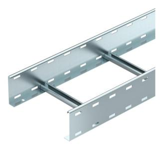
Cable ladder with perforated side rail of side height 110 mm with riveted C profile rungs, open in an upwards direction. The cable ladder is shipped folded up.
