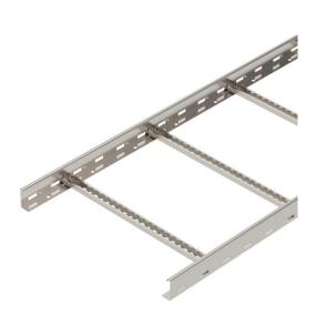
Cable ladder with 60 mm side height with welded C30 profile rungs which are open in an upwards direction. Rolled side rail for reinforcement and as edge protection. Fastening to the bracket takes place using clamps, type LKS 40. The slot dimension of the frame is 16.5 mm and the appropriate clamp clip is type 2056.
