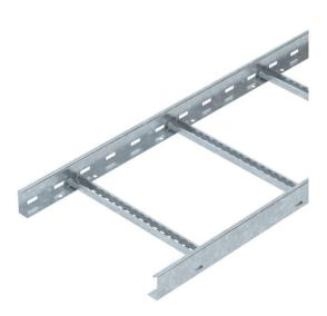
Cable ladder with a 60 mm side height with welded C30 profile rungs which are open in an upwards direction. Rolled side rail for reinforcement and as edge protection. Fastening to the bracket takes place using hold-down clamps, type LKS 40. The slot dimension of the rung is 16.5 mm and the appropriate clamp clip is type 2056.
