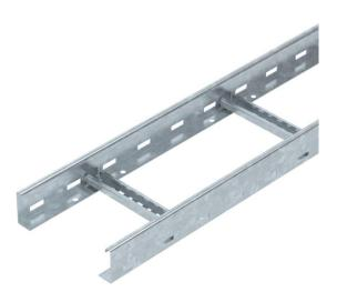
Cable ladder with a 60 mm side height with welded C30 profile rungs which are open in an upwards direction. Rolled side rail for reinforcement and as edge protection. Fastening to the bracket takes place using hold-down clamps, type LKS 40. The slot dimension of the rung is 16.5 mm and the appropriate clamp clip is type 2056.
