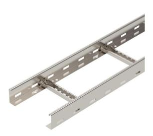
Cable ladder with 60 mm side height with welded C30 profile rungs which are open in an upwards direction. Rolled side rail for reinforcement and as edge protection. Fastening to the bracket takes place using clamps, type LKS 40. The slot dimension of the frame is 16.5 mm and the appropriate clamp clip is type 2056.
