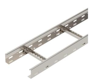
Cable ladder with 60 mm side height with welded C30 profile rungs which are open in an upwards direction. Rolled side rail for reinforcement and as edge protection. Fastening to the bracket takes place using clamps, type LKS 40. The slot dimension of the frame is 16.5 mm and the appropriate clamp clip is type 2056.
