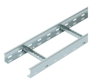
Cable ladder with a 60 mm side height with welded C30 profile rungs which are open in an upwards direction. Rolled side rail for reinforcement and as edge protection. Fastening to the bracket takes place using hold-down clamps, type LKS 40. The slot dimension of the rung is 16.5 mm and the appropriate clamp clip is type 2056.
