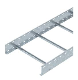
Cable ladder with 110 mm side height with welded C30 profile rungs which are open in an upwards direction. Rolled side rail for reinforcement and as edge protection. Fastening to the bracket takes place using clamps, type LKS 40. The slot dimension of the frame is 16.5 mm and the appropriate clamp clip is type 2056.
