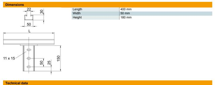
Version for Miscellaneous Maintain electrical functions no Suitable for ceiling fastening yes Suitable for panel fastening no Suitable for profile shapes I profile Rustproof steel, pickled no Angle range, max. 90 mm Angle range, min. 90 mm
