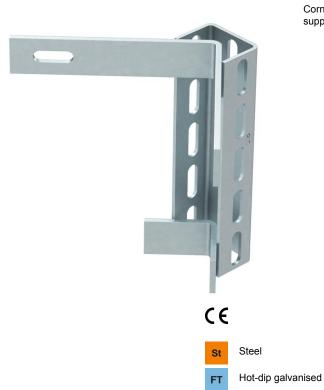
Corner seat with welded U profile for fastening to  $90^\circ$  external corners. Wall and support brackets are screwed to the U profile.
