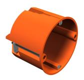
Cavity wall device/connection socket. Dimensions to DIN 49073-1, for plate thickness 7-35 mm. Standard combination spacing 71 mm, option for continuous wiring using connection support for combinations between device sockets and device connection sockets,
