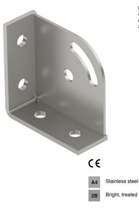
Reinforced mounting bracket with 6 holes to connect profile rails 41 x 41 mm and 41 x 21 mm at an angle of 90°. Additional fastening option for a strut at an angle of 45° with an adjusting range of +/- 30°. Can be used for angles between 15° and 75°.
