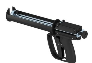
High-quality 2-component cartridge pistol for use with the PYROSIT® NG fire protection foam. The action of the trigger parallel to the handle ensures easy working. Suitable for 5:1 coaxial cartridges. Free the moving parts, push rods and pressure plate from any foam residues and maintain them with a re-greasing cleaning agent.
