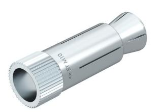
Hollow core anchor "Easy" for mounting in prestressed hollow concrete slabs. When the screw or the nut is tightened, the cone is released from the anchor sleeve and pulled into it. This makes the anchor expand in the hollow space, thereby creating form lock. The hollow core anchor can also be used when the expansion area is not located in the cavity.
