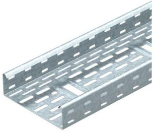
DKS 60 = perforated cable tray system with 60 mm side height. Permeable cable tray system to VdS guideline 2092 with 30% hole surface for use under sprinkler systems.
