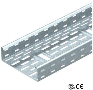
DKS 60 = perforated cable tray system with 60 mm side height. Permeable cable tray system to VdS guideline 2092 with 30% hole surface for use under sprinkler systems.
