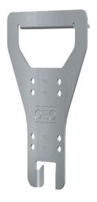
Position the cover lifters as pairs on the cover clamps and remove the chequer plate cover evenly. Repeat lengthways until the entire cover is removed. Alternatively, the cover lifter can be used as a template for the connector perforation with cable trays cut during construction. For this, turn the cover lifter through 180° and position on the cable tray. Then use the perforation template appropriate to the side height.
