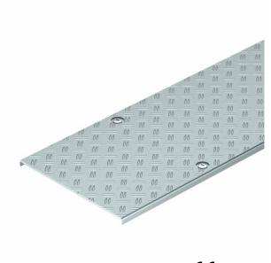
Cable tray cover for the walkable BKRS cable tray system. The basic cover is strip galvanised in a material thickness of 2 mm with additional aluminium chequer riveted on in a thickness of 4 mm, sturdy and non-slip. Turn buckle fastening with a turn buckle distance of 500 mm.
