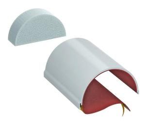
Internally coated half shell, the inner space of which can be fully assigned with cables and electrical installation pipes. For interior application. CE-labelled, European approved construction product according to ETA-13/0904 and German general type approval. Fire resistance up to 120 minutes.
