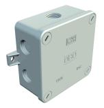
Protection rating IP67, empty box for use with individual terminals, four plastic cover screws, thus absolute corrosion-protection, two fastening bases for screws of up to 5 mm  $\emptyset$ , 7 break-out entries with thread M20 x 1.5. 3 polyamide cable glands for cable diameters of 9–12 mm, type 106 M.
