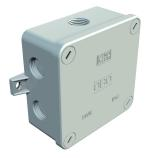
B 9 K ...: Protection IP67 Empty box to be used with single terminals 4 cover screws of plastic, so fully corrosion-proof 2 fixing holes for screws up to 5 mm diameter 7 breakout entries with Pg 16 thread, with 3 cable glands of polyamide for cable diameters of 10–14 mm type 106/16 B9K The cable glands have a specially shaped thread which automatically breaks out the entry when the gland is screwed in.
