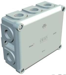
Protection rating IP54, nominal voltage 660 V, nominal cross-section  $10 \div mm^2$ , two fastening holes for screws up to 6 mm Ø on the outside of the box, four cover screws, 10 break-out entries with thread M20 x 1.5, primarily for cable glands with short connecting thread.
