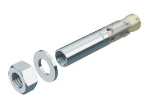
Bolt tie BZ-IG with internal thread for the anchoring of medium-duty to heavy-duty loads, both in cracked and non-cracked concrete. It combines high approved loads with small edge distances and axial spacings. Undercutting the drill holes is not necessary.
