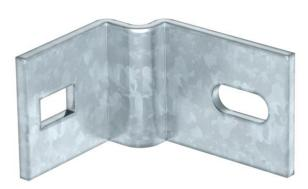
Mounting angle for mounting IS 8 supports on the wall. The mounting angle can also be used in conjunction with the heavy-duty vertical ladder, type SLS 80. Including fastening bolt M12x30. Including truss-head bolt M12 x 30.
