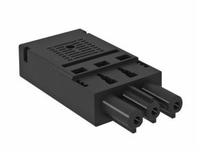
Socket part, 3-pin, type GST18i with spring power connection for rigid cables of 1.5–2.5 mm², single-wire and ultrasonically welded, fine wire cables 1.5 mm² with end sleeves, unmounted with strain relief, can be terminated in situ, 250 V, 16 A.
