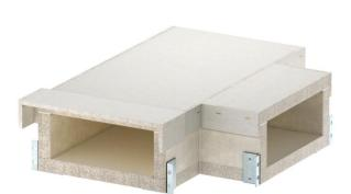
T piece for PYROLINE® Con S BSK I90/E30 fire protection duct, consisting of fibreglass lightweight concrete which is resistant to water and frost, for the creation of T branches of the duct. Mounted connectors ensure quick mounting in situ, whilst loosely placed covers ensure quick inspection and reassignment.
